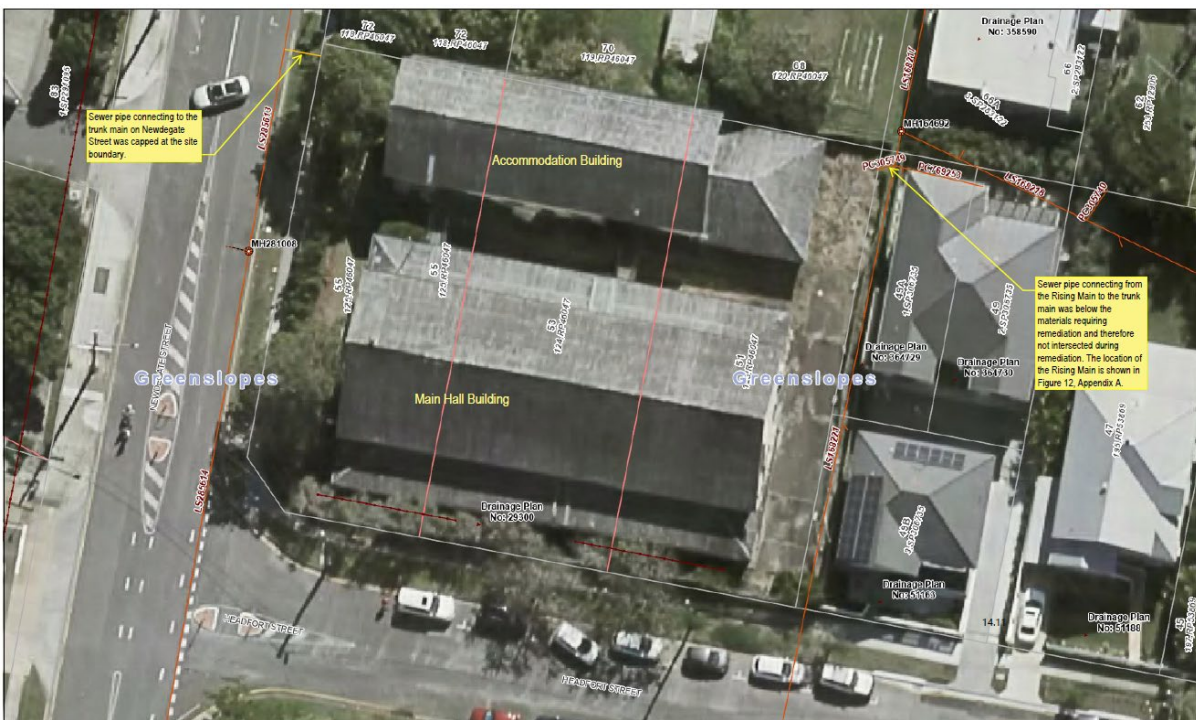
Plate 5. Layout of infrastructure removed during remediation including the sewer pipes on the northeast and north west site boundaries
